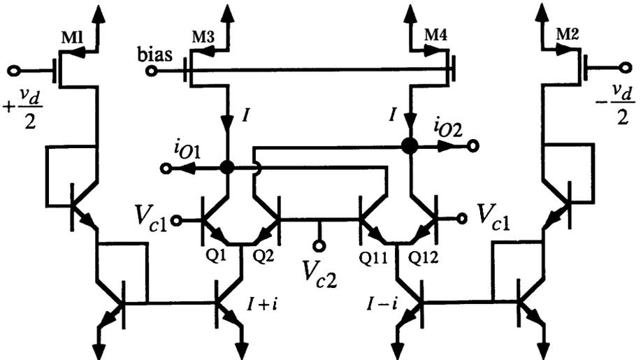
Fig. 2. The basic transconductor illustrating tuning mechanism.
