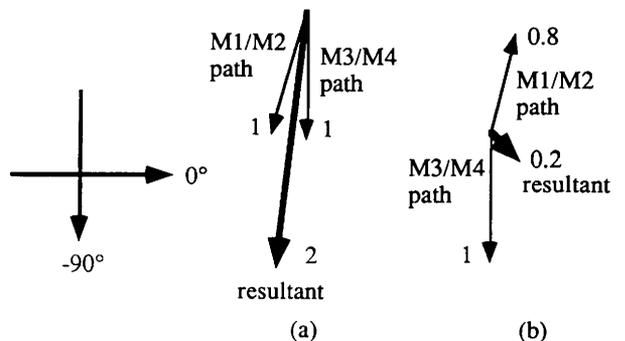
Fig. 5. Illustrating magnitude and phase of output signal for two possible  $G_m$  settings. (a) maximum  $G_m$ ; (b)  $0.2G_{m,max}$ .
