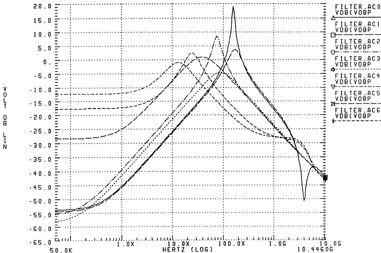
Fig. 10. Bandpass function frequency response for various  $f_o$  and  $Q$  settings.
