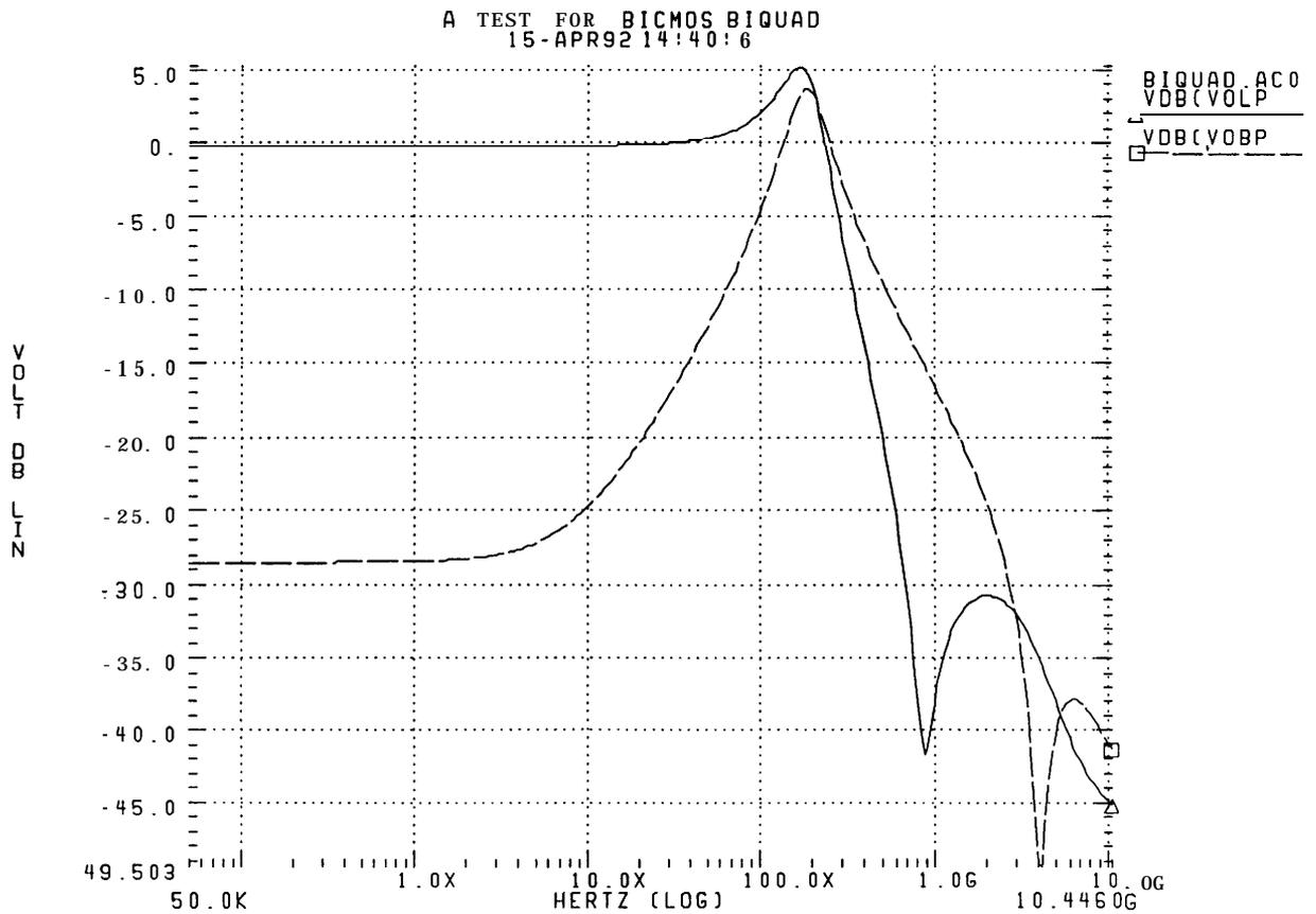
Fig. 8. Illustrating the effects of transconductor excess damping on biquad frequency response.
