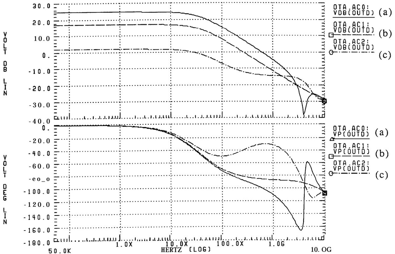
Fig. 6. OTA frequency response for a setting of (a) maximum  $G_m$ , (b)  $0.5G_m$ , (c) a low value for  $G_m$ .
