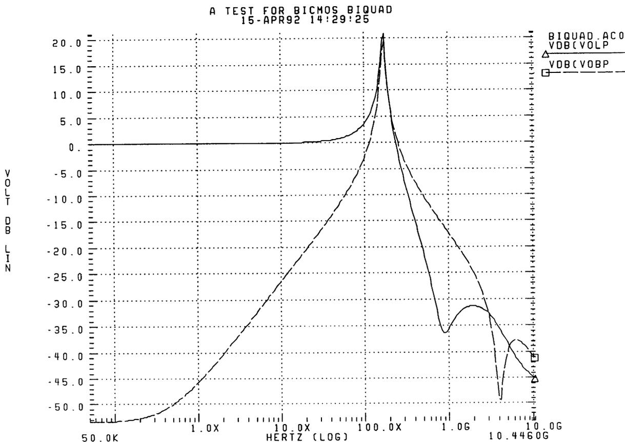
Fig. 9. Biquad frequency response showing the effects of feedforward and Q-enhancement.
