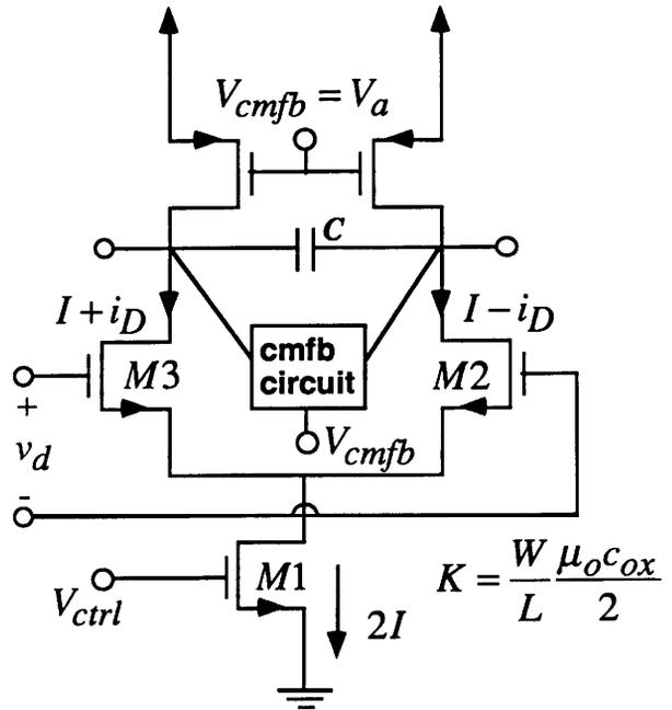
Fig. 1. A simple tunable transconductor integrator.
