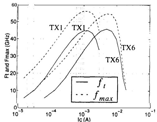
Fig. 2. Measured  $f_t$  and  $f_{max}$  versus  $I_C$  for both TX1 and TX6 transistors at  $V_{CE} = 1$  V.
