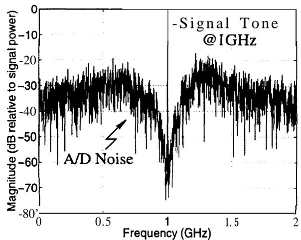
Fig. 8. Simulated output spectrum of a fourth-order LC bandpass modulator.
