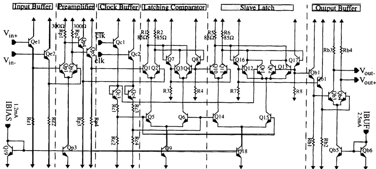
Fig. 3. A complete schematic of the SiGe HBT return-to-zero comparator
