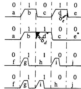
Fig. 1. Illustration of NRZ nonlinearity. (a) NRZ (0 1 0 1 0) pattern. (b) NRZ (0 1 1 0 0) pattern. (c) RZ (0<sub>1</sub> 0<sub>1</sub> 0<sub>1</sub>) pattern. (d) RZ (0<sub>1</sub> 1<sub>1</sub> 0<sub>1</sub>) pattern.
