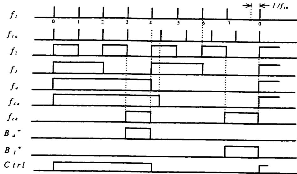
Figure 5.23 Timing diagram in the timing recovery circuit
